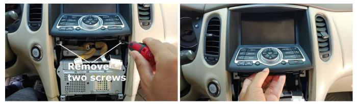
5. Remove the 2 screws on the metal brackets below the display screen and then remove the screen assembly after disconnecting the 3 connectors behind it.
