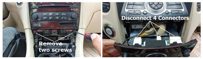
4. Remove the 2 screws below the bezel/control panel buttons. Then gently wiggle & pull it toward you to remove that section.
