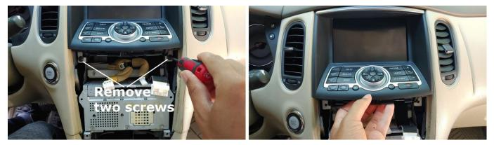
5. Remove the 2 screws on the metal brackets below the display screen and then remove the screen assembly after disconnecting the 3 connectors behind it.
