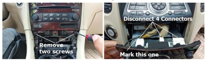
4. Remove the 2 screws below the bezel/control panel buttons. Then gently wiggle & pull it toward you to remove that section. G37 cars trim bezel would also have the a/c vents on it.
