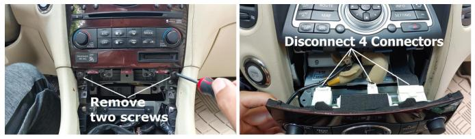
4. Remove the 2 screws below the bezel/control panel buttons. Then gently wiggle & pull it toward you to remove that section.
